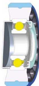
roller with cover and cover washer (CCW)
