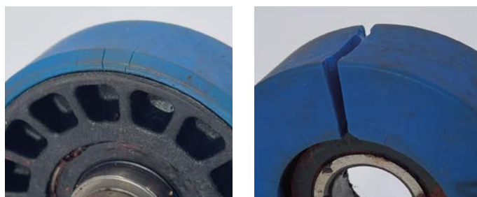
Damage caused to non-hydrolysis-resistant rollers after immersion in water for 1,000 hrs at 80° C
