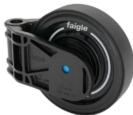
The plastic wheel shaft is so stable that it significantly exceeds the load-bearing capacity of the ball bearing. Fitted in damping bushings, the wheel shaft is securely attached by inserting it into the fork from the underside. This can be done by hand, with no tools required.
