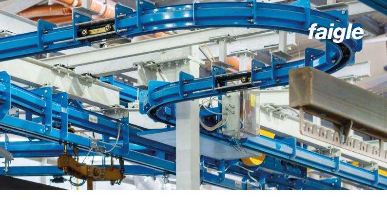
faigle's overhead conveyor carriages feature specially designed smooth-running ball bearings with a contact-less cover plate. A range of special high-performance plastics with excellent smooth-running properties, outstanding wear resistance and effective noise insulation qualities are available for the tyre. Enclosed tyres mounted on the outside of the carriage, which protects the ball bearing against dust and other environmental influences, are another option.
